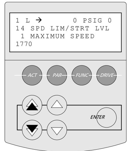
**Minimum Speed** - As the demand on the pump decreases, PumpSmart will decrease the pump speed to match the new demand. This Minimum Speed parameter sets the minimum speed that the pump can operate at. It is also used to define the safe speed to run the pump during a pump protection fault. The default value for minimum speed is 25% of 11.07 MOTOR FL RPM.
