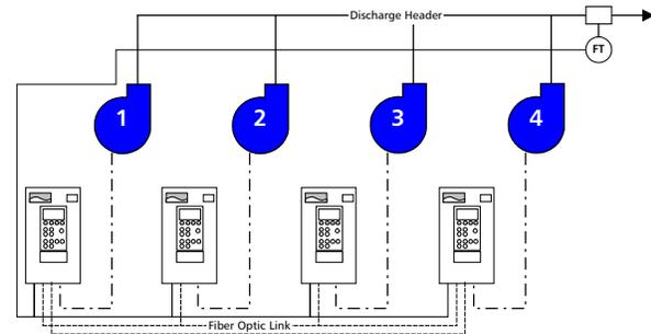
**Figure 2 - Single Process Transmitter Configuration TX ONE AI** – Where each PS200 is wired in series with a single process transmitter.
