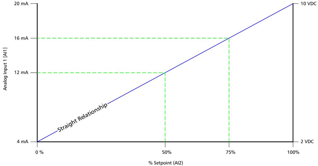
The effect is a straight relationship with the maximum setpoint value corresponds to the maximum signal [i.e. 20 mA or 10 VDC] while the minimum setpoint value corresponds to the minimum signal [4mA or 2 VDC].
