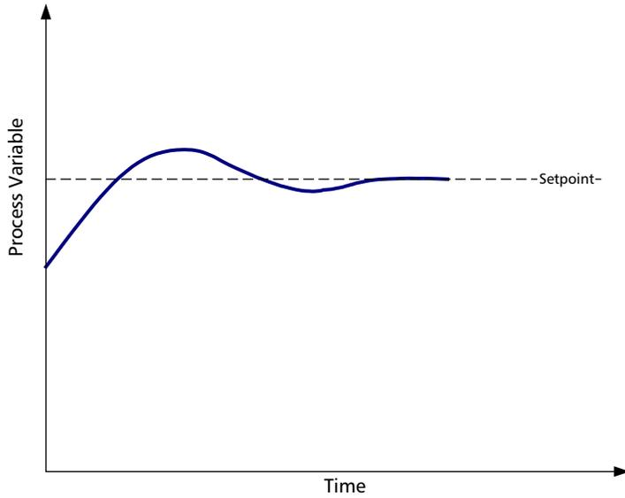
**Under-Compensated system:** In this case, the drive is under-compensating to the error in the setpoint. The integration time in this case is too long.
