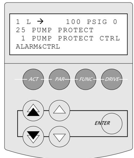
**NOTE** - The PumpSmart keypad will display an alarm or fault message "Pump Protect" when the protection limit condition exists. The Pump Protection feature may also be configured to warn via DCS [optional Fieldbus module] or sonic or visual alarms through the digital relay output. See **OPTIONS** for details.
