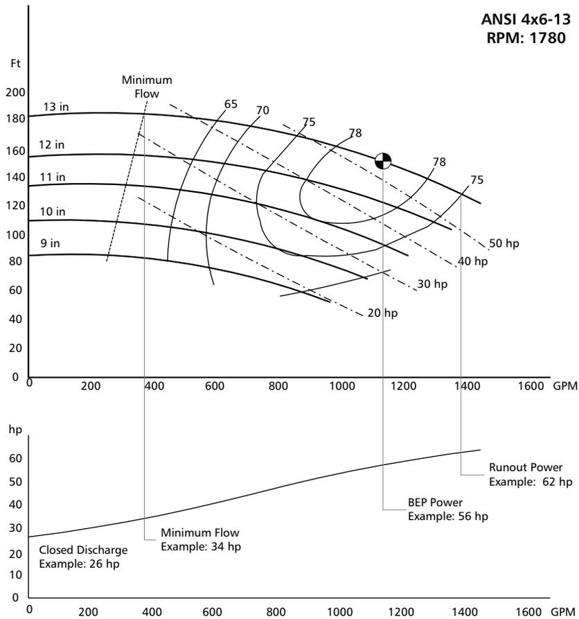
**NOTE - Application of the Torque Pump Protect functionality is limited to pumps having power curves that are constantly rising from a closed valve operating condition. These pumps are typically with specific speeds of 2000 or under.**
