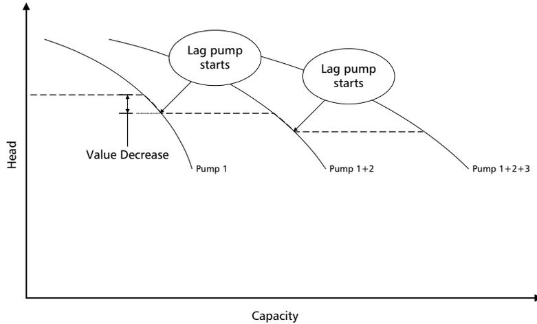
22.02 VALUE DECREASE - The above figure shows a constant pressure system where Pump 2 is started when Pump 1 cannot maintain the constant pressure and it drops by the amount shown as VALUE DECREASE.
