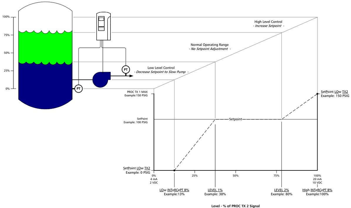
*EXAMPLE – In the above diagram, the setpoint is 100PSIG. When the second process transmitter (TX2) is below 38% of its signal, it will begin to scale back the setpoint linearly from 100 PSIG to 0 PSIG (occurs at 13% of its signal). When the second process transmitter (TX2) reaches 79% of its signal, it will increase the setpoint linearly from 100 PSIG to 150 PSIG at 100% of signal*
