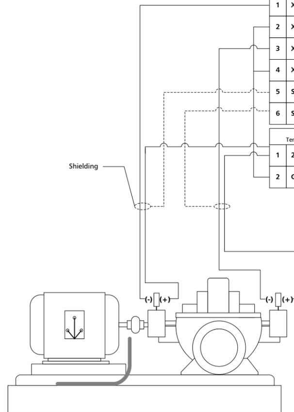
Example: Double Suction Pump With 2 Vibration Transmitters
