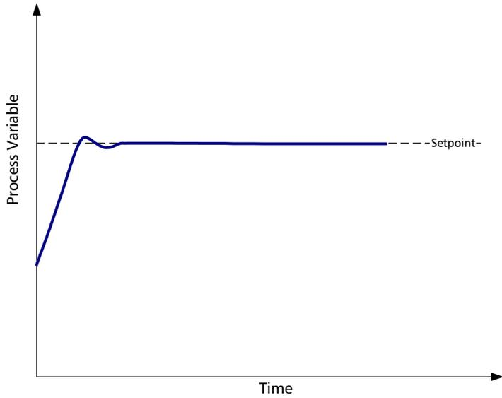
**Tuned system:** This system tuning is also acceptable. There is a slight overshoot to the setpoint, however the response rate is better than the previous "Normally Tuned" system.
