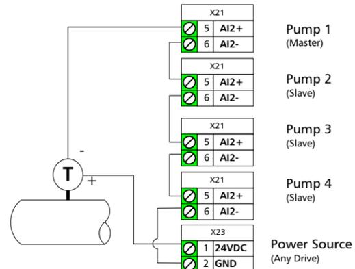
**PumpSmart Powered Transmitter**
