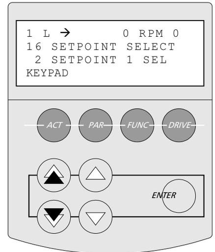
**NOTE - SETTING AI2 MAX (16.03) AND AI2 MIN (16.04) IS STILL REQUIRED IF USING KEYPAD OR FIELDBUS CONTROL**
