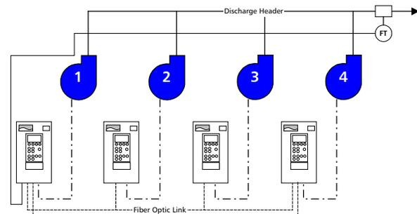
**Figure 3 - Single Process Transmitter Configuration TX ONE MASTER** – Where the process transmitter is wired into the MASTER PS200 and the process signal is communicated to the slave PS200 units via the fiber optic cable..
