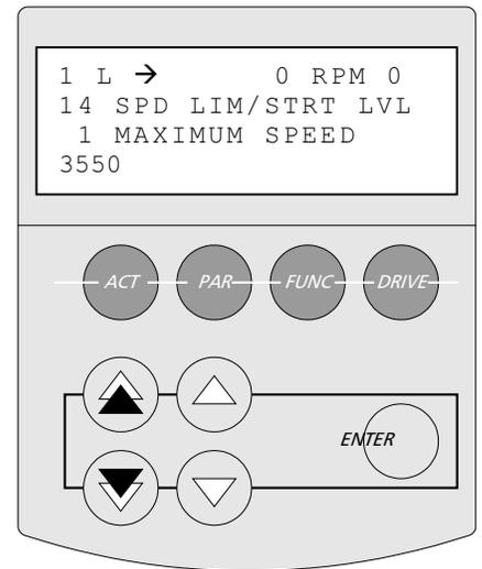
**Minimum Speed** - The Minimum Speed parameter sets the minimum speed that the pump can operate at. It is also used to define the safe speed to run the pump during a secondary pump protection fault if the pump protection is programmed this way. The default value for minimum speed is 25% of 11.07 MOTOR FL RPM
