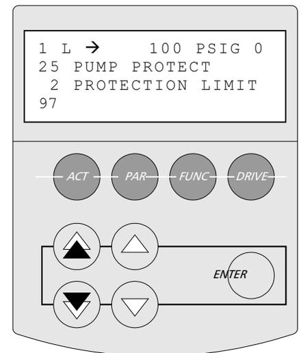
**NOTE** - A delay can be set so that the PumpSmart PS200 waits to respond if the process variable falls below the protection limit. This will prevent the PumpSmart unit from shutting down prematurely due to momentary system upsets. See the OPTIONS section for further detail.
