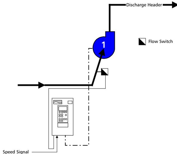
**Figure C - Speed Control Secondary Protection**
