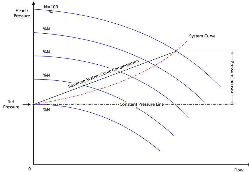
In this case the system pressure setpoint is shown at shutoff and the increase in setpoint pressure is shown for increasing flow.
