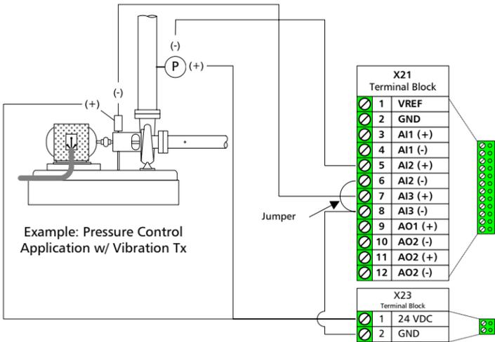
Example: Pressure Control Application w/ Vibration Tx
