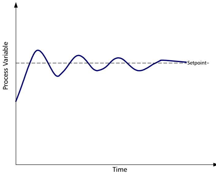
**Over-Compensated system:** In this case, the drive is over-compensating to the error in the setpoint resulting in an oscillation. The proportional gain is too high and the integration time is too short.
