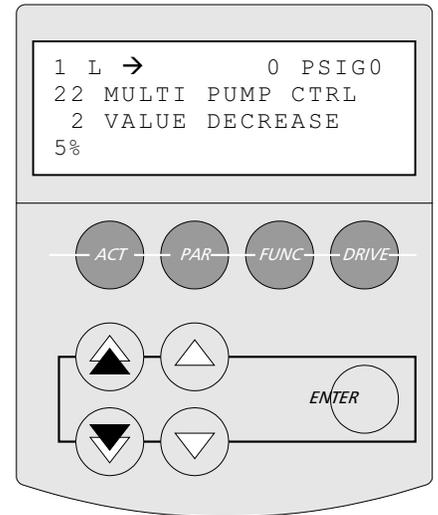
22.03 VALUE INCREASE - As shown in previous figure, the actual process setting will decrease by the VALUE DECREASE with each additional pump that is added. To compensate for this the VALUE INCREASE parameter increases the setpoint for each pump that is added.
