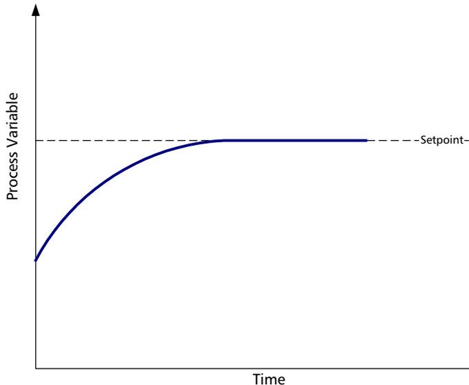
**Normally tuned system:** This system has appropriate gain and integration times resulting in a smooth transition towards the setpoint.
