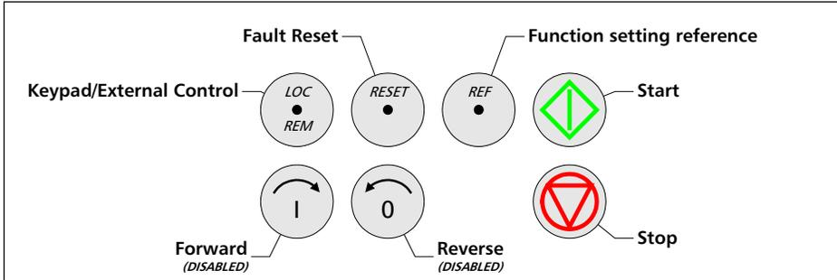
All operational commands such as start, stop and Setpoint can be given pressing the appropriate key on the keypad when the control location is local. This is indicated by an L (Local Control) in the upper left hand corner of the status row.
