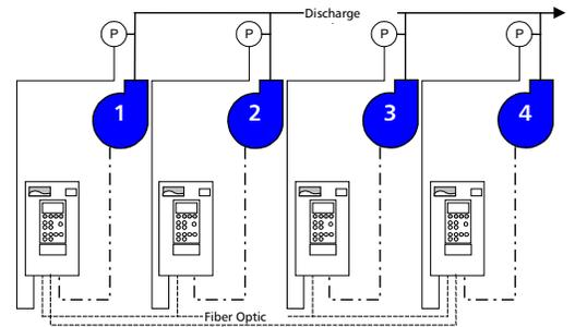
**Figure 1 - Typical Multi-Pump Configuration TX ALL DRIVES** – Where each PS200 has its own pressure transmitter
